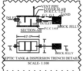
SEPTIC TANK & DISPERSION TRENCH DETAIL SCALE: 1:100
